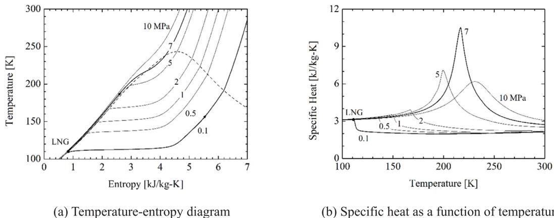
Fig. 2. Thermodynamic properties of typical LNG (with a composition of 91% methane, 5% ethane, 2% propane, 1% butane, and 1% nitrogen on mole basis) at different pressure levels.
