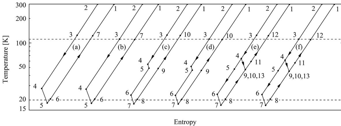
Fig. 9. Temperature-entropy diagram of optimized cycles: (a) standard with HP LNG (b) standard with LP LNG (c) 2-stage with HP LNG (d) 2-stage with LP LNG (e) dual-turbine with HP LNG (f) dual-turbine with LP LNG.
