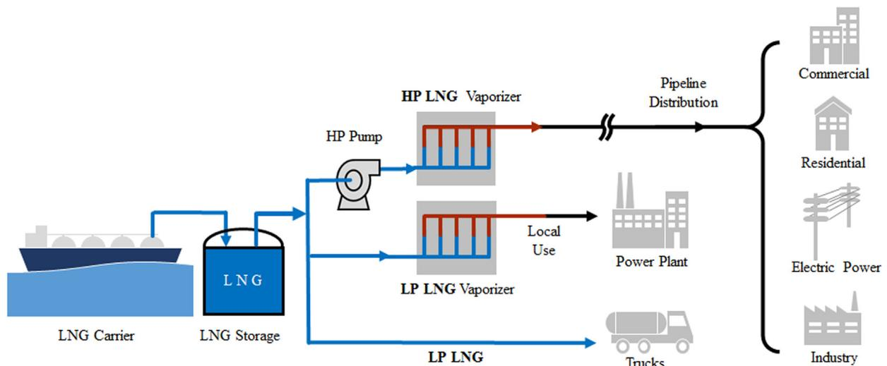
Fig. 1. Schematic illustration of LNG supply process where the cold energy is utilized at two pressure levels: high-pressure (HP) for pipeline distribution and low-pressure (LP) for local use or truck delivery.
