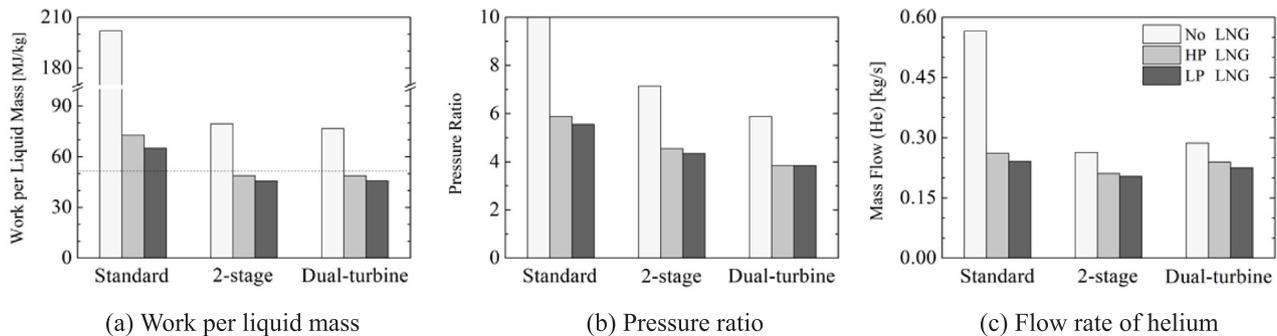
Fig. 10. Comparison of optimized cycles with or without LNG pre-cooling.
