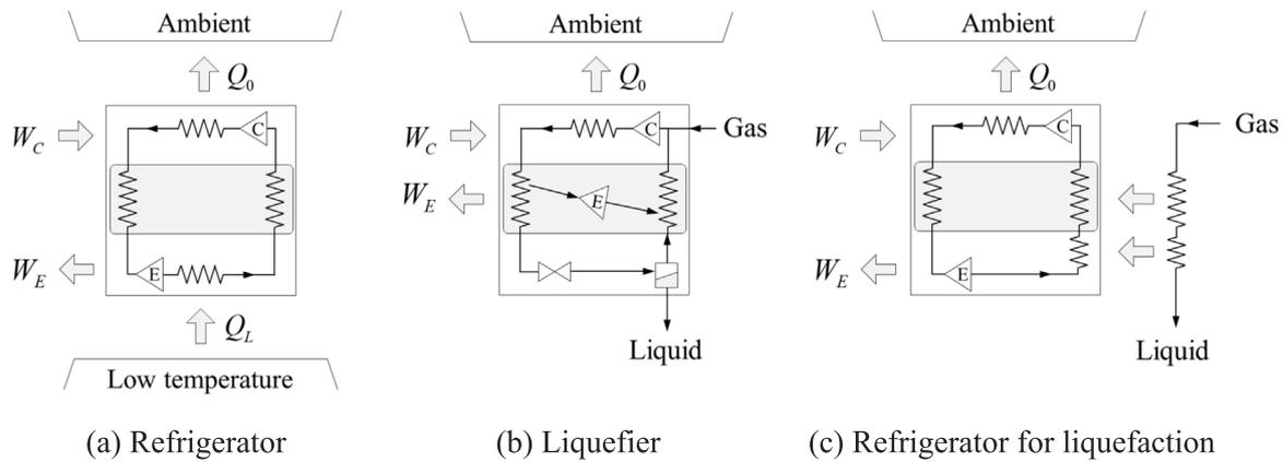
Fig. 3. Comparison of thermodynamic cycles for refrigeration and liquefaction: (a) closed-cycle Brayton refrigerator, (b) open-cycle Claude liquefier, and (c) closed-cycle Brayton refrigerator for liquefaction.
