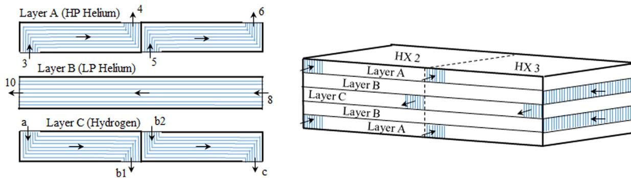
Fig. 12. An example of schematic configuration for plate-fin heat exchanger (PFHX) to combine HX2 and HX3 with three different layers (A, B, C) by A-B-C-B-A stack (not to scale).
