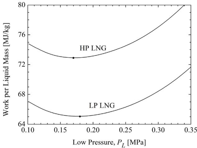
Fig. 6. Work per liquid mass as a function of  $P_L$  in LNG pre-cooled standard cycle.
