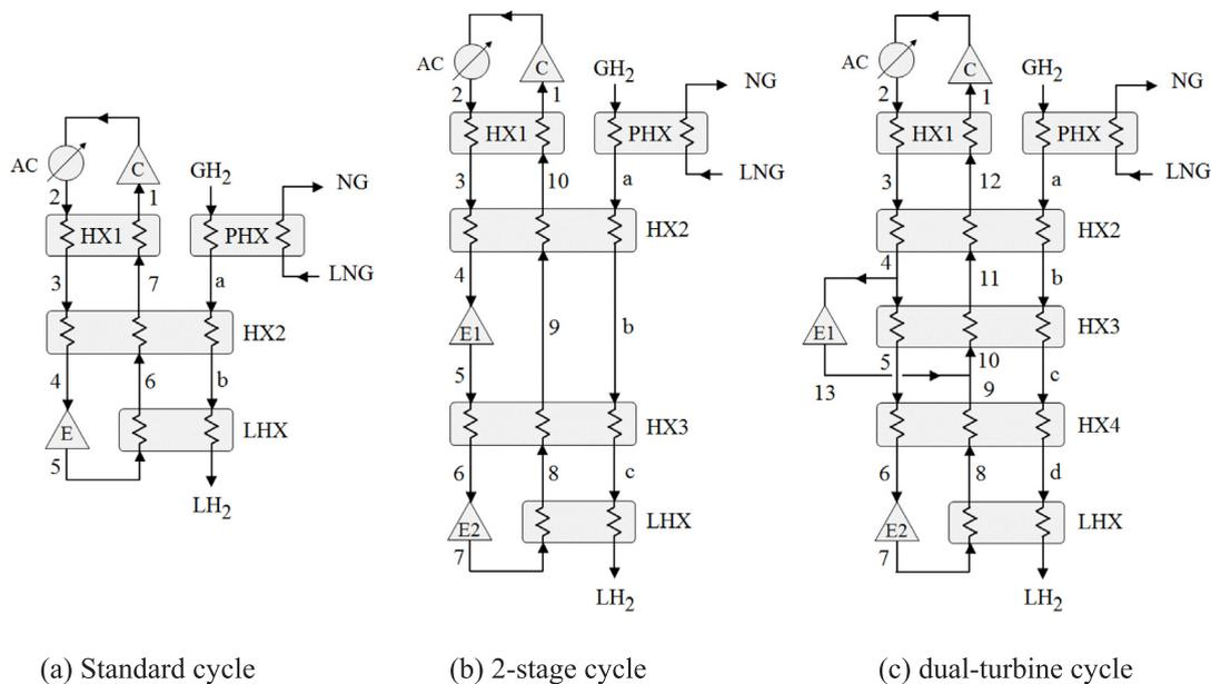
Fig. 4. Standard and two modified Brayton refrigeration cycles for liquefaction with LNG pre-cooling.
