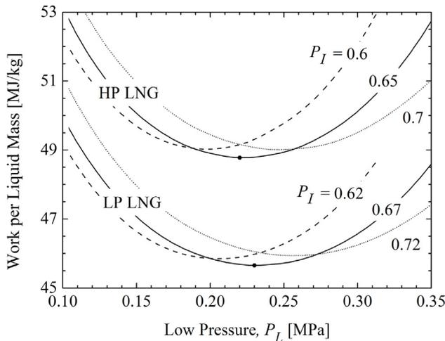
Fig. 7. Work per liquid mass as a function of  $P_L$  for various values of  $P_I$  in LNG pre-cooled 2-stage cycle.
