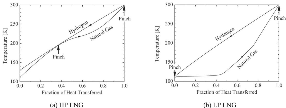
Fig. 5. Comparison of temperature profile in pre-cooling heat exchanger (PHX) with HP LNG and LP LNG.
