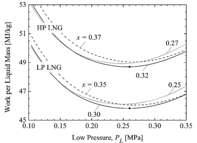
Fig. 8. Work per liquid mass as a function of pressure ratio for LNG pre-cooled dual turbine cycle.
