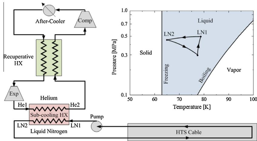
Fig. 1. Cryogenic refrigeration system for HTS power cable and liquid-nitrogen cycle on phase diagram.
