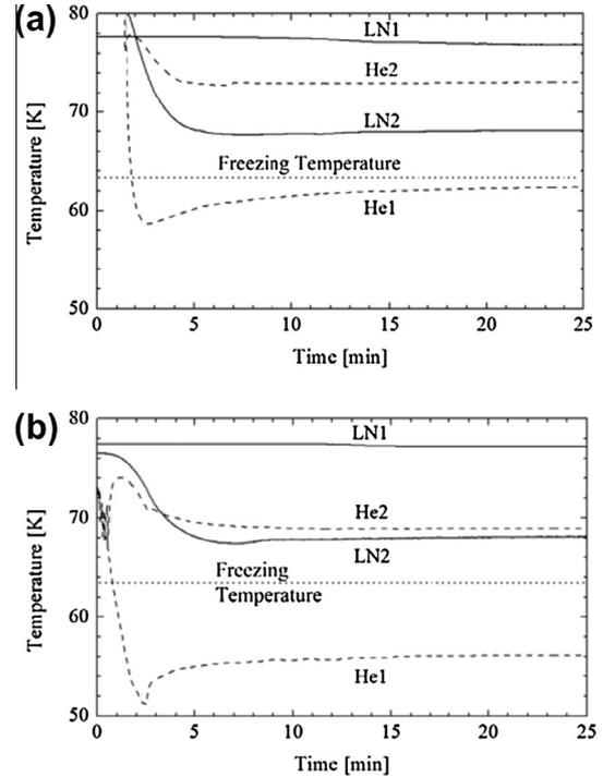
Fig. 8. Measured temperature history to obtain a steady-state for sub-cooling liquid nitrogen from 77.4 to 68.0 K. (a) Counter-flow HX. (b) Two-pass cross-flow HX.
