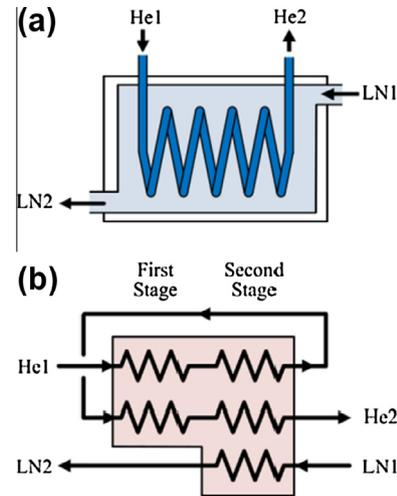
Fig. 3. Anti-freezing schemes presented by Yoshida et al. [9]. (a) Tube-in-bath type. (b) Two-stage type.
