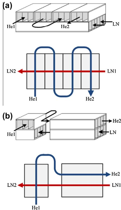
Fig. 10. Ideas to improve the effectiveness of cross-flow heat exchangers. (a) Multi-pass cross-flow HX. (b) Combined cross-flow and counter-flow HX.
