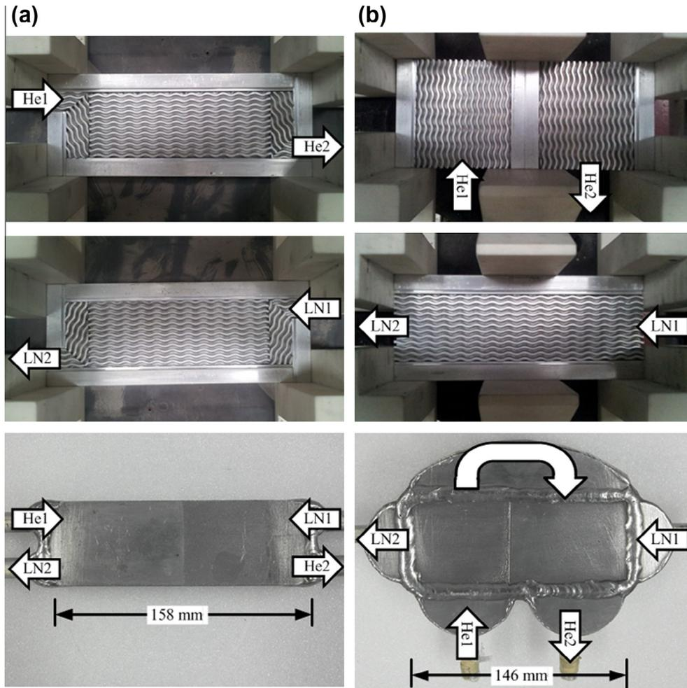
Fig. 5. Layer-by-layer and assembled photographs of test heat exchangers. (a) Counter-flow. (b) Two-pass cross-flow.
