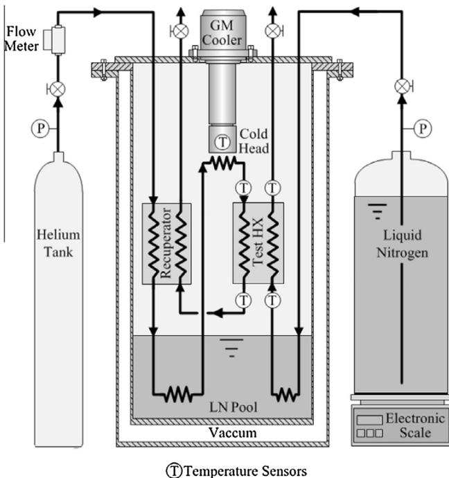
Fig. 6. Schematic overview of experimental set-up.
