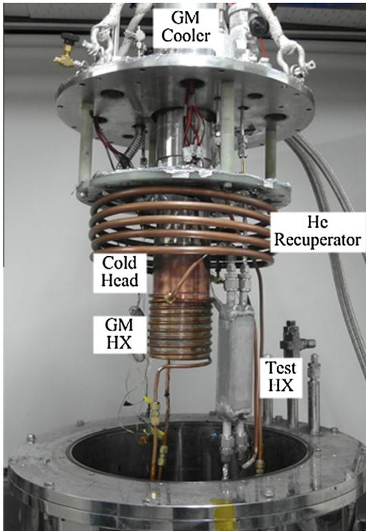
Fig. 7. Photograph of top-plate assembly of cold-head, helium recuperator, GM heat exchanger, and test heat exchanger.
