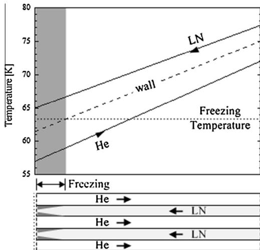
Fig. 2. An example of temperature profile in sub-cooling heat exchanger under freezing condition.
