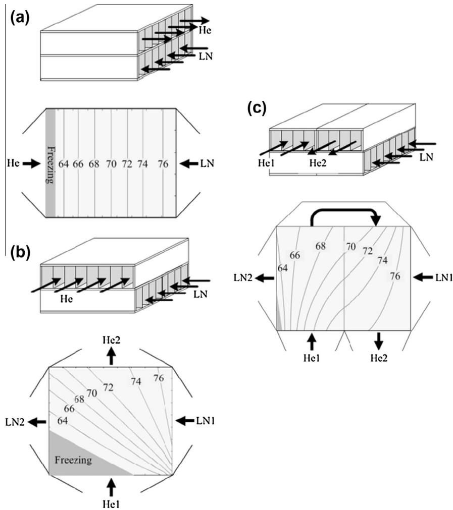
**Fig. 4.** Configuration of plate-fin heat exchangers and typical isotherms to illustrate the freezing area. (a) Counter-flow heat exchanger. (b) Cross-flow heat exchanger. (c) Two-pass cross-flow heat exchanger.
