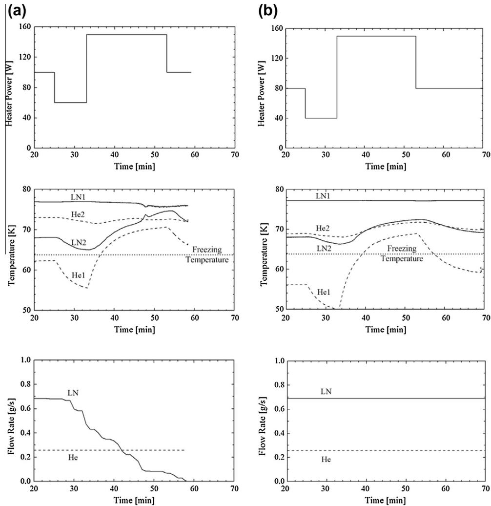
Fig. 9. Stepwise variation of heater power to cold-head of cryocooler, and measured history of temperature and flow rate. (a) Counter-flow HX. (b) Two-pass cross-flow HX.
