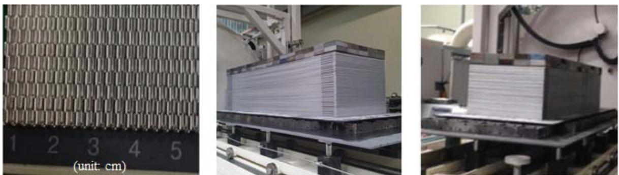
Fig. 5 Photographs of serrated fins and stacked plate-fins for brazing.
