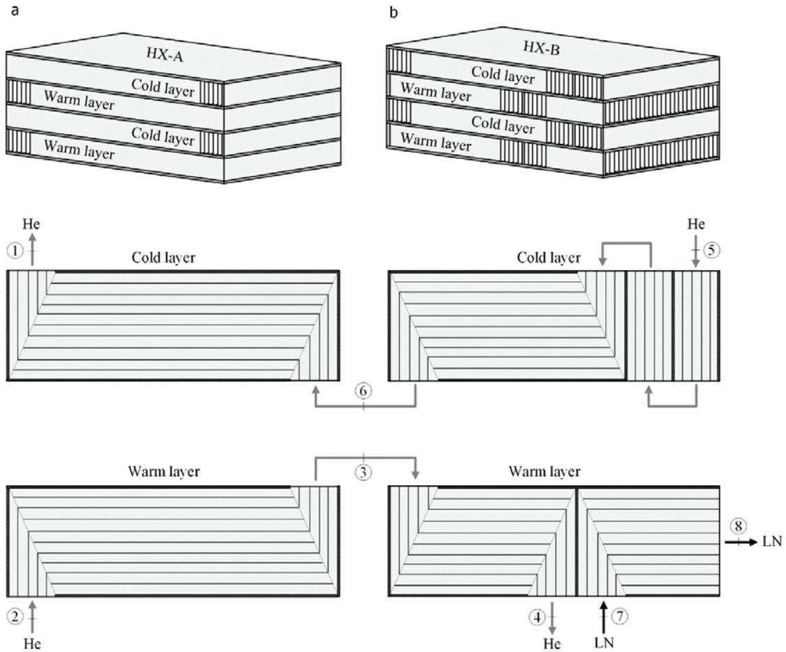
Fig. 3. Graphic representation of plate-fin heat exchanger design (a) HX-A (b) HX-B.
