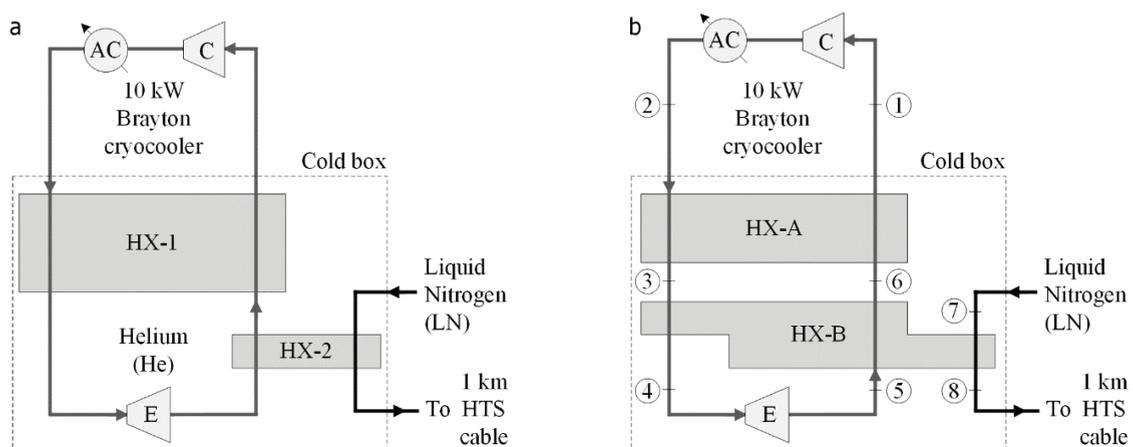
Fig. 1. Schematic flow diagram of cryogenic cooling system for a 10 kW Brayton cryocooler and a 1 km HTS cable (a) basic cycle (b) modified cycle with integrated HX design (C: compressor, AC: after-cooler, E: expander, HX: heat exchanger, He: helium, LN: liquid nitrogen).
