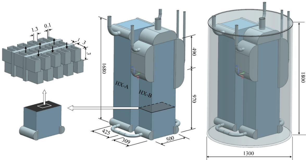
Fig. 4 Three-dimensional drawings of plate-fins and heat exchanger assembly (unit: mm).
