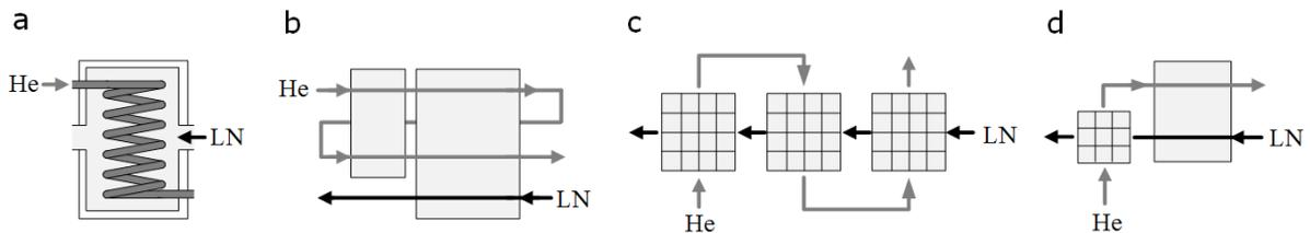
Fig. 2. Schematics of four different anti-freezing schemes proposed by Yoshida et al. [7] and Chang et al. [9] (a) tube-in-bath HX; (b) two-stage HX; (c) multi-pass cross-flow HX; (d) combined cross-flow and counterflow HX.
