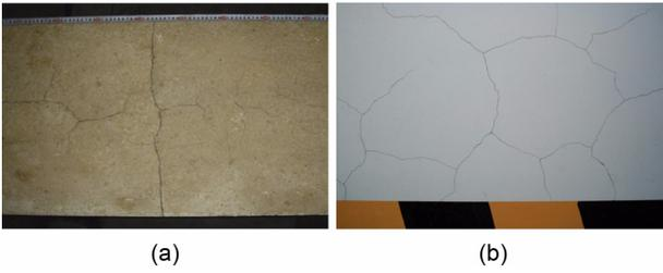
Fig. 1 Radial cracks caused by biaxial stress state on concrete surface
