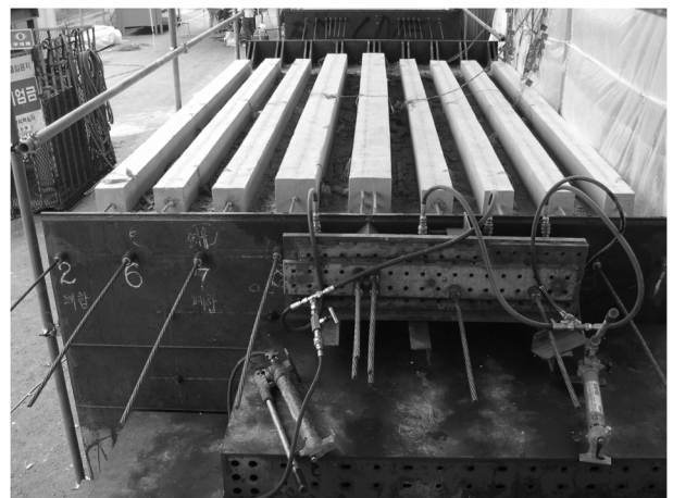
Fig. 4 Testing members and prestressing frame
